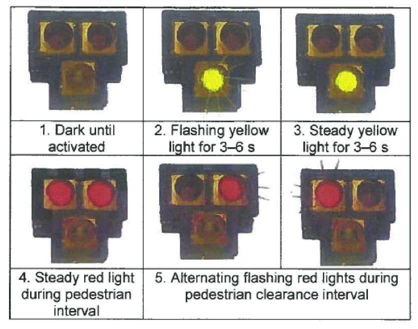
Figure 3. Chart. Example of phase sequence for a HAWK. (2)
